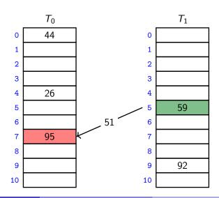
M = 11,  $h_0(k) = k \mod 11,$   $h_1(k) = \lfloor 11(\varphi k - \lfloor \varphi k \rfloor) \rfloor$
