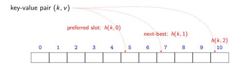
Simplest method for open addressing: *linear probing*  $h(k,j) = (h(k) + j) \mod M$ , for some hash function *h*.
